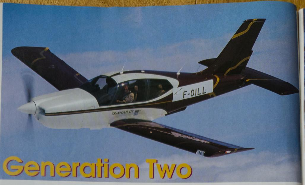
GTs. The updated version I fly for this test will eventually take the new Morane Renault diesel engines, but at present is still powered by the Lycoming IO-540. F-OILL is awaiting collection from Biggin Hill by its new owner and will spend its life in the Middle East—the French registration is only temporary.
