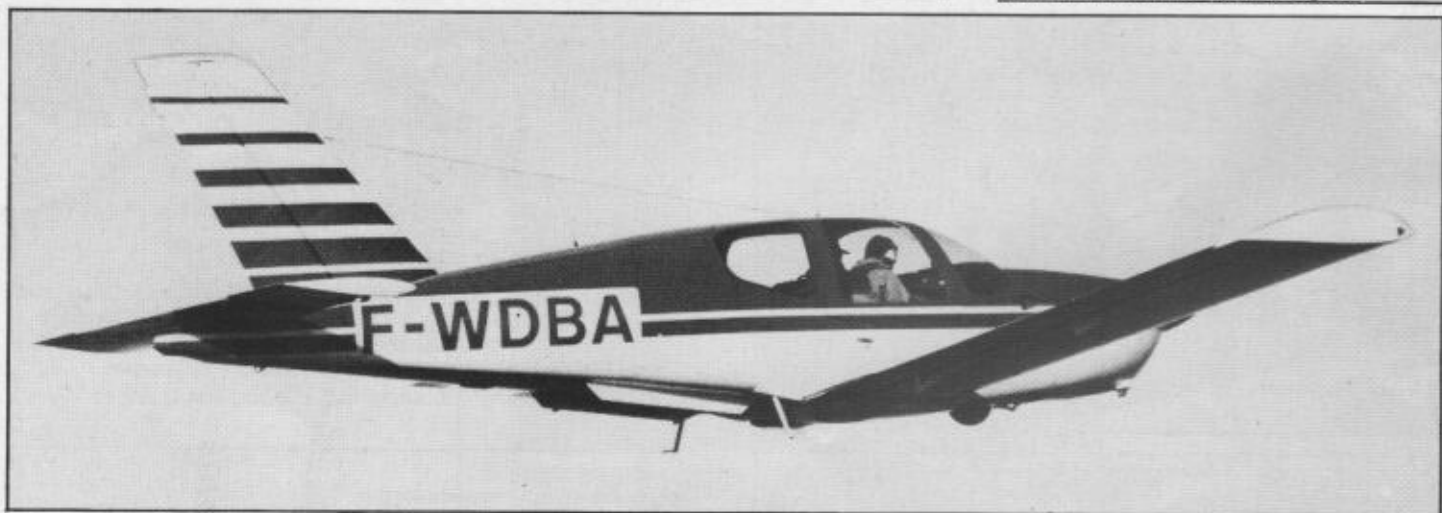
Tampico (left) and Tobago (above) are externally indistinguishable. The Tampico has a 160-hp Lycoming driving a fixed-pitch prop; the Tobago 180-hp and constant-speed. Coming soon is the Trinidad (below) with 235-hp and retractable gear.
