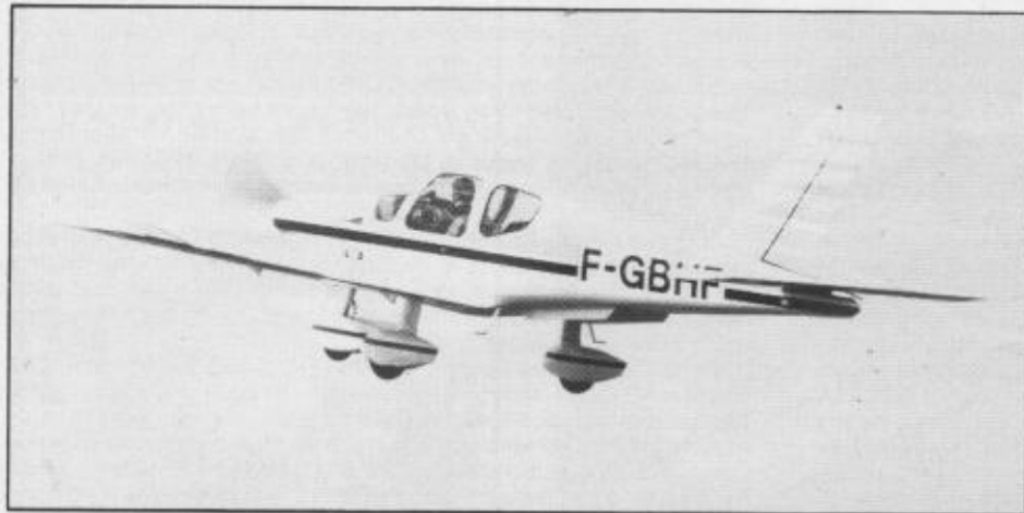
Tampico (left) and Tobago (above) are externally indistinguishable. The Tampico has a 160-hp Lycoming driving a fixed-pitch prop; the Tobago 180-hp and constant-speed. Coming soon is the Trinidad (below) with 235-hp and retractable gear.
