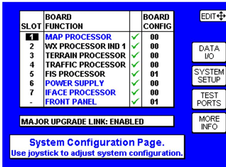
FIGURE 4-107 System Configuration Page With Slot 5 As ‘FIS PROCESSOR’
