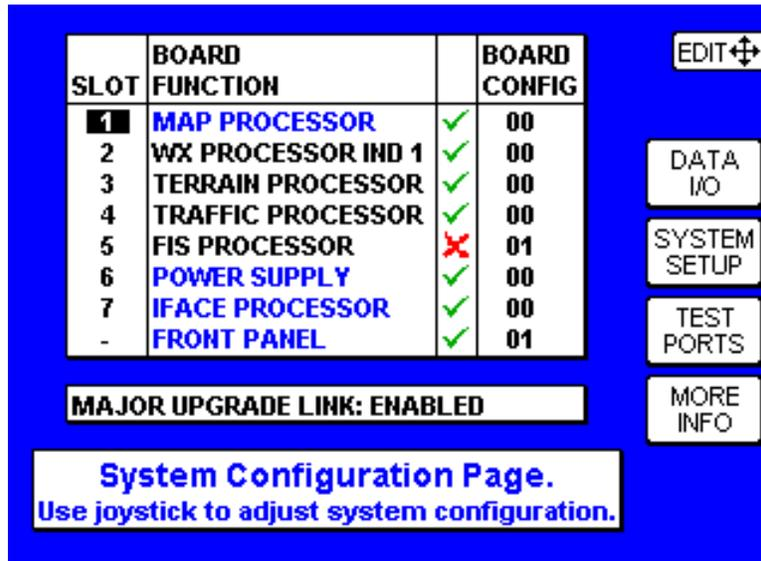
FIGURE 4-108 System Configuration Page With 'FIS PROCESSOR' Fault
