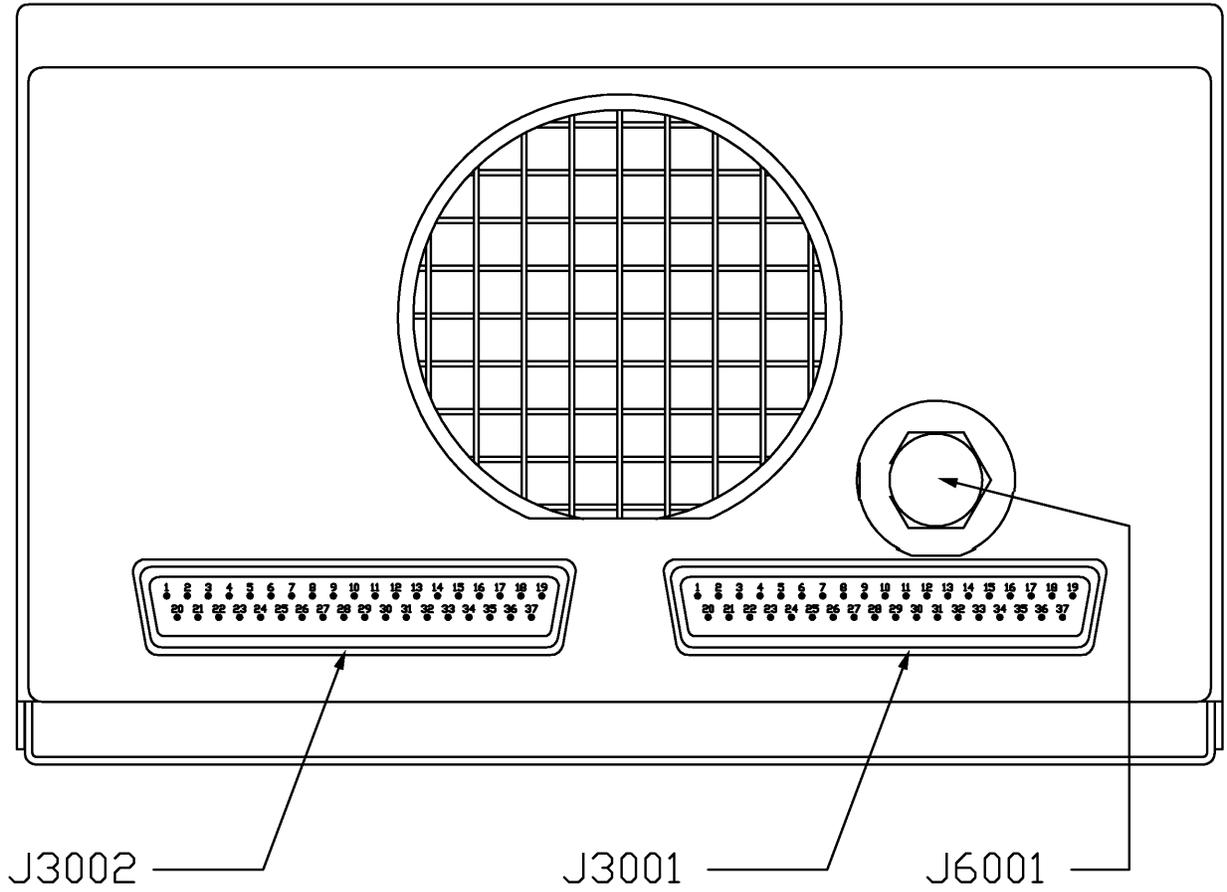
FIGURE 2-1 KMD 540 Exploded Rear Connector Diagram
