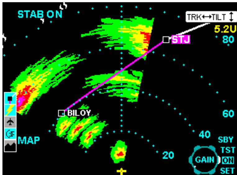
FIGURE 4-57 WX Horizontal Profile View In Ground Mapping Mode
