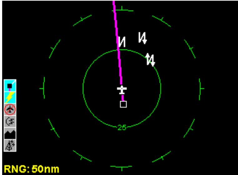
FIGURE 4-128 WX-1000E (Stormscope) 360 Degree View
