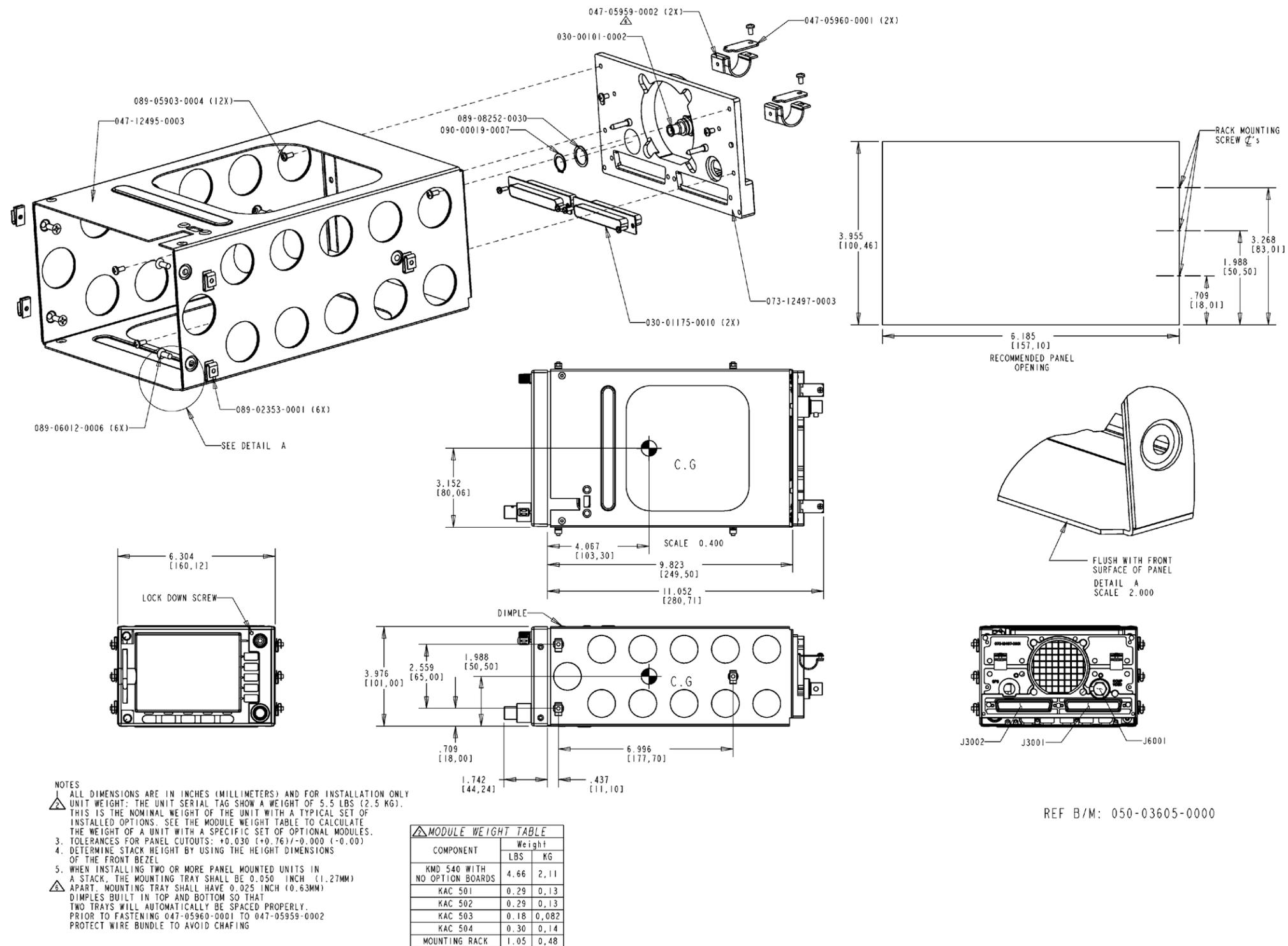
FIGURE 2-5 KMD 540 Installation Drawing (P/N 155-06053-0000 Rev. F)
