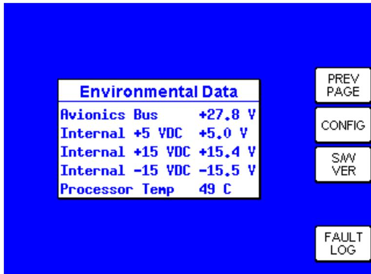
FIGURE 4-72 WX-500 Stormscope System Data Option, Environmental Data Page
