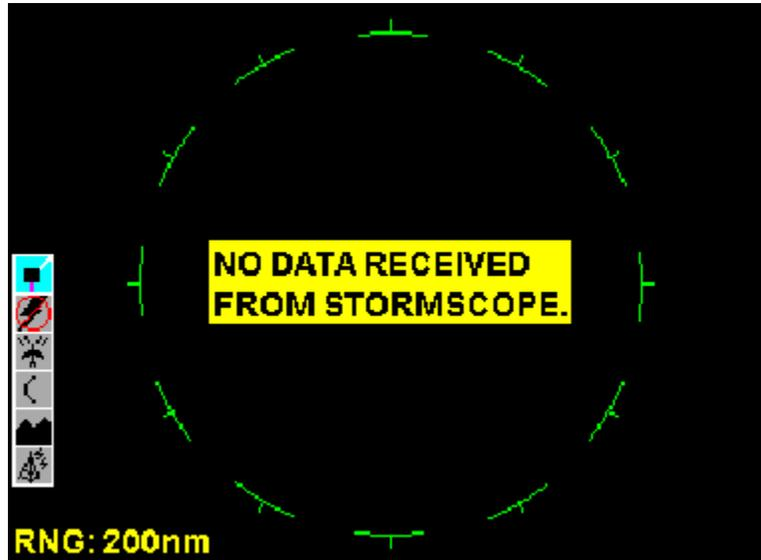
FIGURE 4-127 WX-1000E (Stormscope) Display with Fault Message
