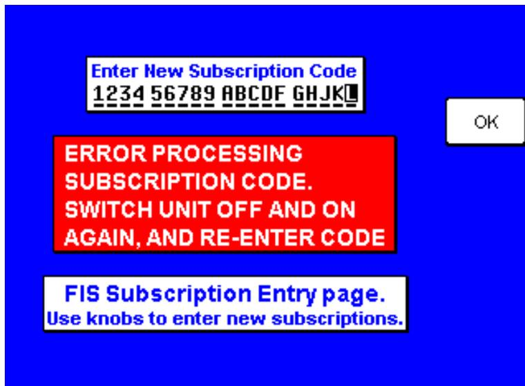
FIGURE 4-119 Subscription Processing Fault
