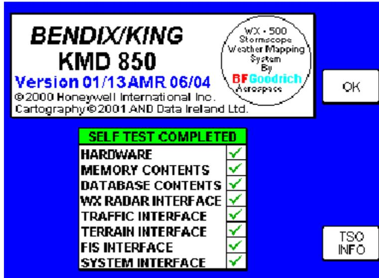
FIGURE 4-53 WX Radar Interface Self Test Passed
