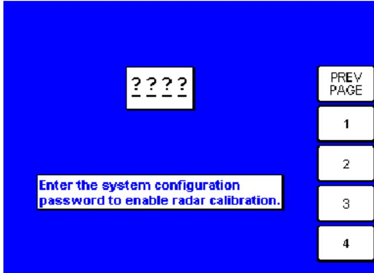
FIGURE 4-50 KMD 540 Radar Configuration Password Page
