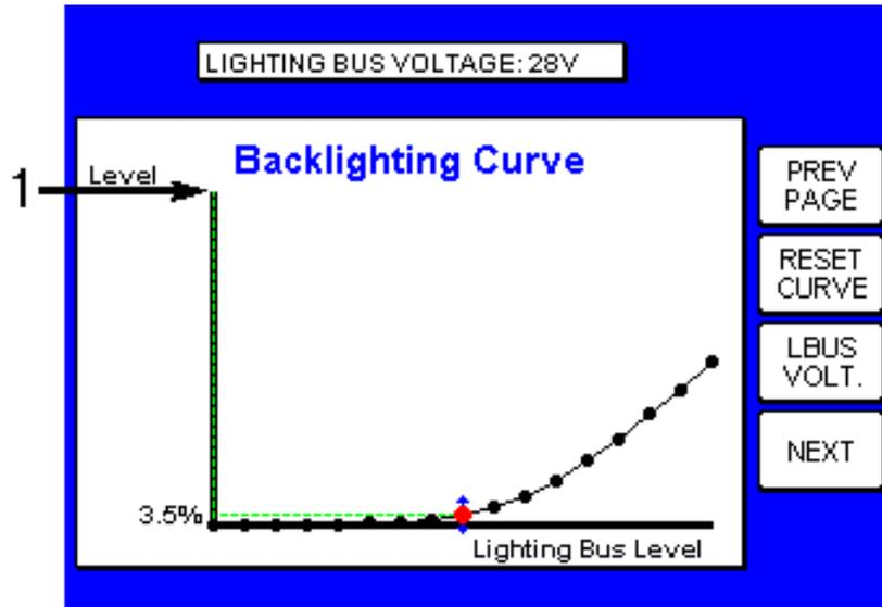
1. Lighting Bus Level Input (relative to the Aircraft’s Lighting Bus Control)
