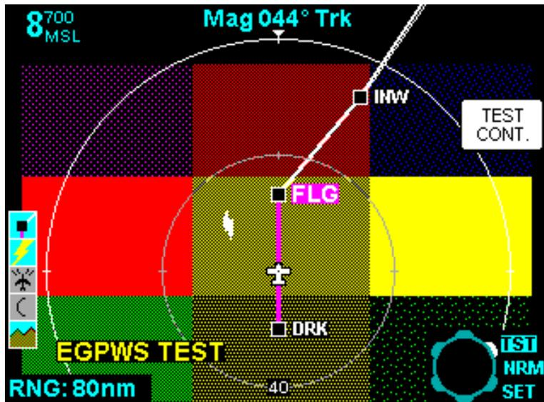
FIGURE 4-83 EGPWS Self Test Page With Rotary Control
