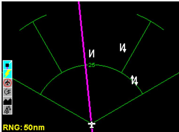
FIGURE 4-129 WX-1000E (Stormscope) 120 Degree View
