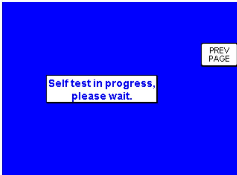
**FIGURE 4-74 WX-500 Stormscope Self Test In Progress Page**
