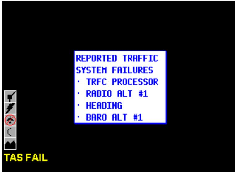
FIGURE 4-105 Traffic System Faults Page
