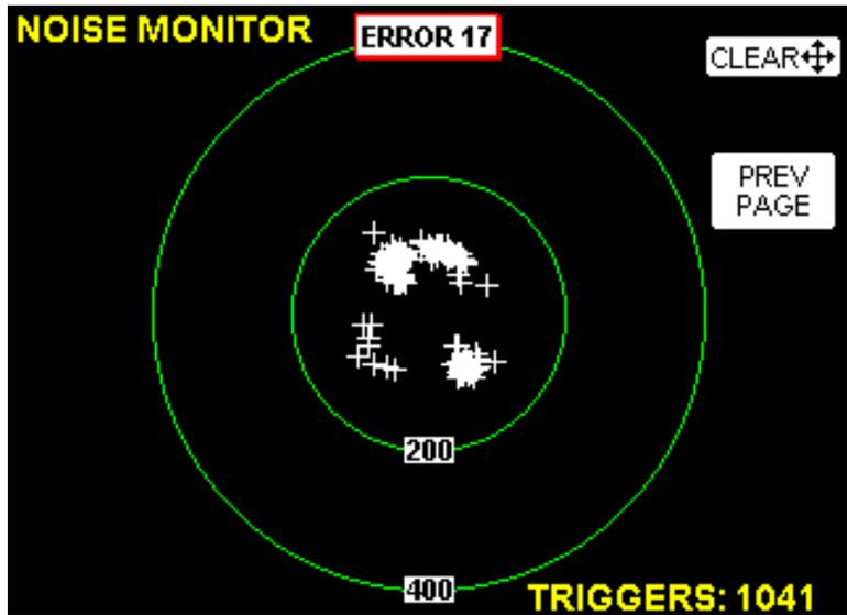
FIGURE 4-68 WX-500 Stormscope Noise Check
