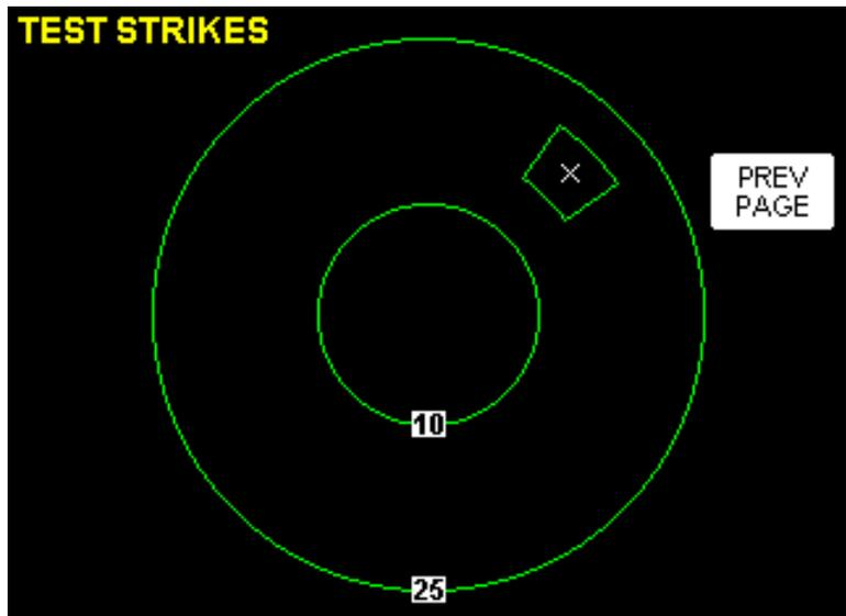
FIGURE 4-69 WX-500 Stormscope Strike Test
