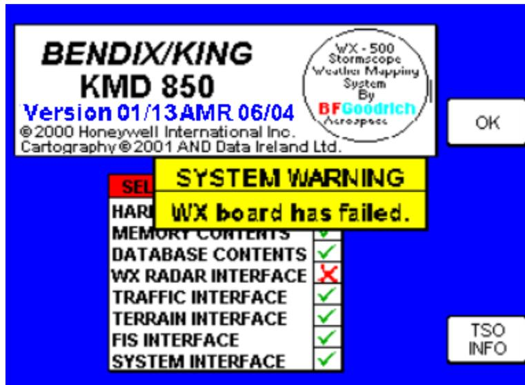
FIGURE 4-54 WX Radar Interface Self Test Failed
