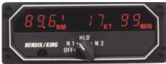
Fig 3. Honeywell KDI 572 remote distance annunciator. Cost of unit plus interface, installation and approval: approx €7000
