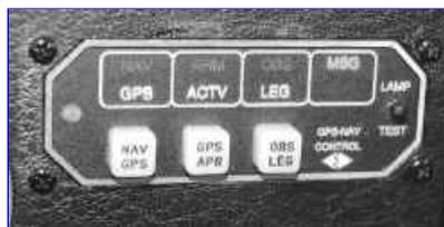
**Two must-have items for most GPS IFR installations include a TSO'd antenna, top, and a remote annunciator / switching panel, such as the MD41, lower photo. Some navigators have self-contained annunciation.**
