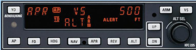
automatically disconnected when excessive pitch and roll rates or excessive acceleration forces are sensed. Well-placed voice messages and audible warnings keep pilots alert to the environment around them. When the system is powered up, an extensive pre-flight test automatically inspects the monitors and other components of the system to ensure proper operation.
