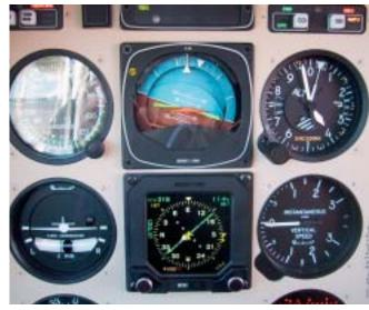
the display changes to a LOC annunciation. When a localizer with glideslope is tuned, glideslope symbology appears down the right side of the display directing vertical guidance.
