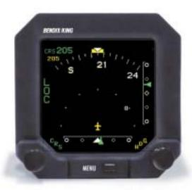
In the GPS Map mode (previous page), the KI 825 depicts flight plan waypoints and route along with lightning data. In the localizer mode (left), a glideslope indicator appears on the right side of the display. The GPS HSI mode (right) shows a full compass rose. The white arrow in the bottom left of the image points to the tuned VOR.
