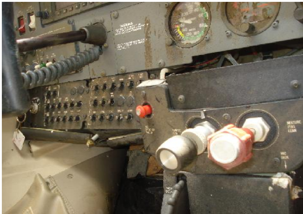
THROTTLE FULL & MIXTURE LEAN, KEY ON BOTH(MAG)
