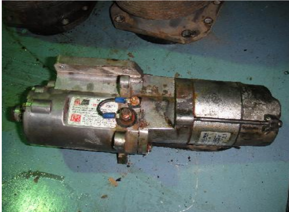
STARTER SHOWING SIGN OF OVERHEAT
