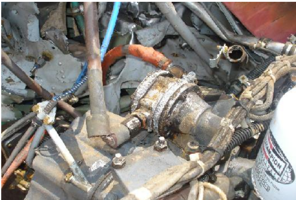
FUEL DISTRIBUTION VALVE WITH BURN MARK
