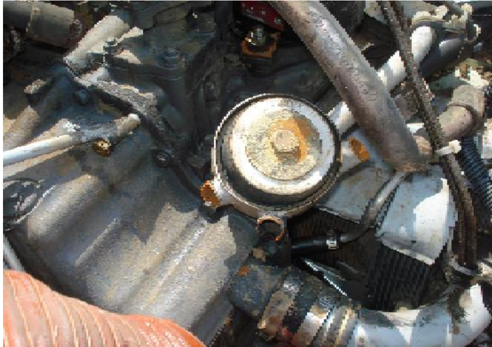
BLACK SOOT ON EXHAUST & ON ENGINE
