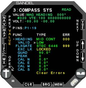
The Compass System page configures the gyro and fluxgate (if applicable) to the SN3500.
