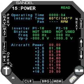
Monitors power inputs to the SN3500 including the #1 and #2 inverters.
