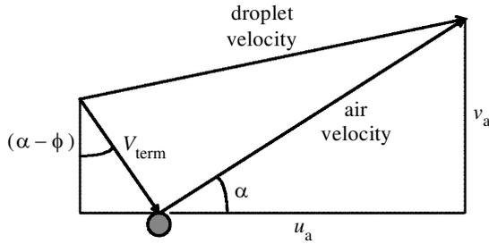
Figure 6. Determination of initial droplet velocity.
