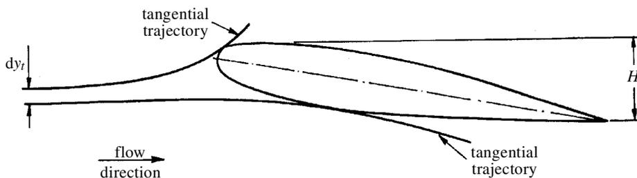
Figure 8. Definition of the overall catch efficiency,  $E = dy_t / H$ .
