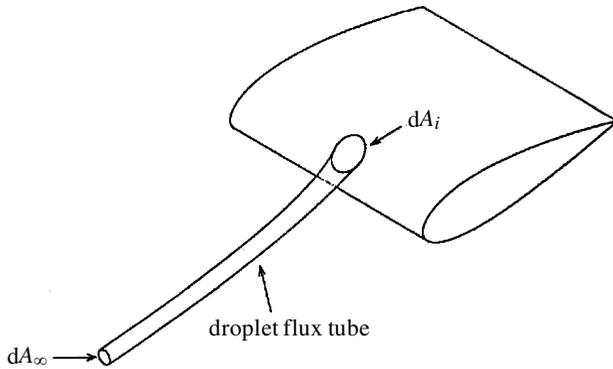
Figure 9. Definition of the local catch efficiency on a three-dimensional geometry,
