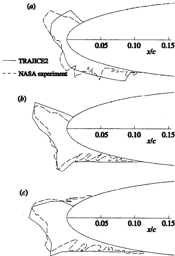
Figure 14. Example of typical spread in accuracy achievable with ice-accretion prediction codes. Incidence is  $4^{\circ}$ , airspeed is  $94\text{ m s}^{-1}$ , VMD is  $20\text{ }\mu\text{m}$ , LWC is  $1.05\text{ g m}^{-3}$ , time is 6.2 min. (a)  $t = -6.6\text{ }^{\circ}\text{C}$ ; (b)  $t = -12.2\text{ }^{\circ}\text{C}$ ; (c)  $t = -16.6\text{ }^{\circ}\text{C}$ .
