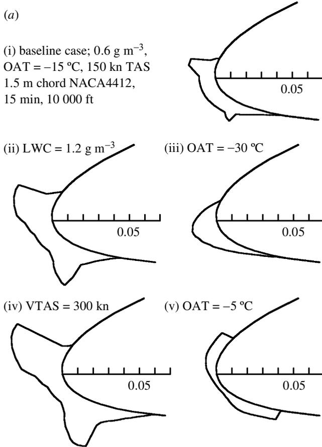
Figure 13. (a) Illustration of the effect of key parameters on the ice-accretion profile.
